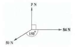
A body is in equilibrium under the action of three focuses,  $P\,N$ ,  $50\,N$  and  $84\,N$  as shown in the diagram. What is the magnitude of P?
