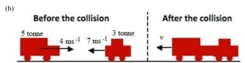
Velocity of coupled trucks =  $0.125 \text{ ms}^{-1}$ Direction is the same as the three-tonne truck.
